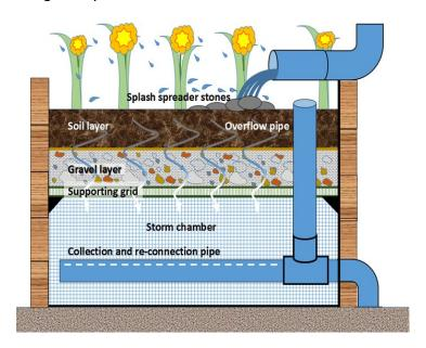
Example of a Raingarden attached the down pipe of a building
